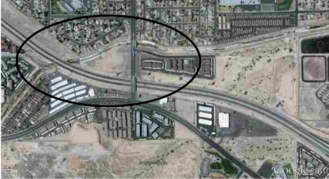
Figure 14: Reverse curve located on US 95 and Russell Rd interchange, curve with smaller radius circled
